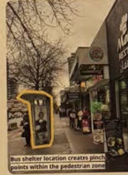
Bus shelter location creates pinch points within the pedestrian zone.
